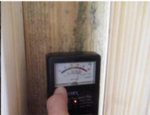
Moisture stains with microbial-like growth visible at several areas. Areas tested wet using a moisture meter.
