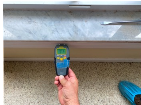
Visible stain(s) tested wet, using a moisture meter. This indicated active moisture was present. Unable to determine underlying condition.
